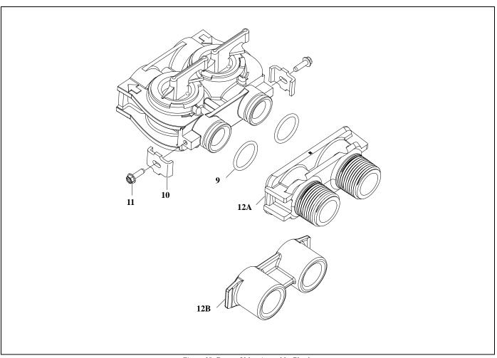
Figure 18: Bypass Valve Assembly, Plastic
