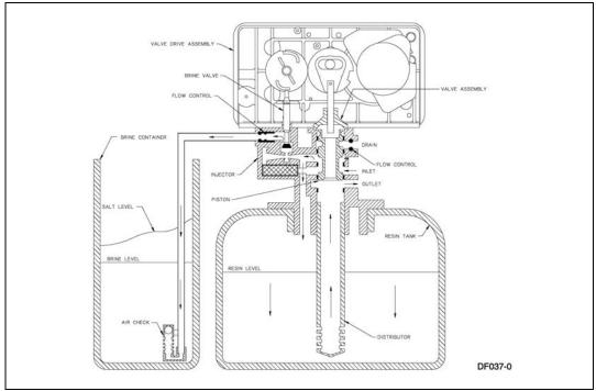
Figure 13: Brine Tank Fill Position
