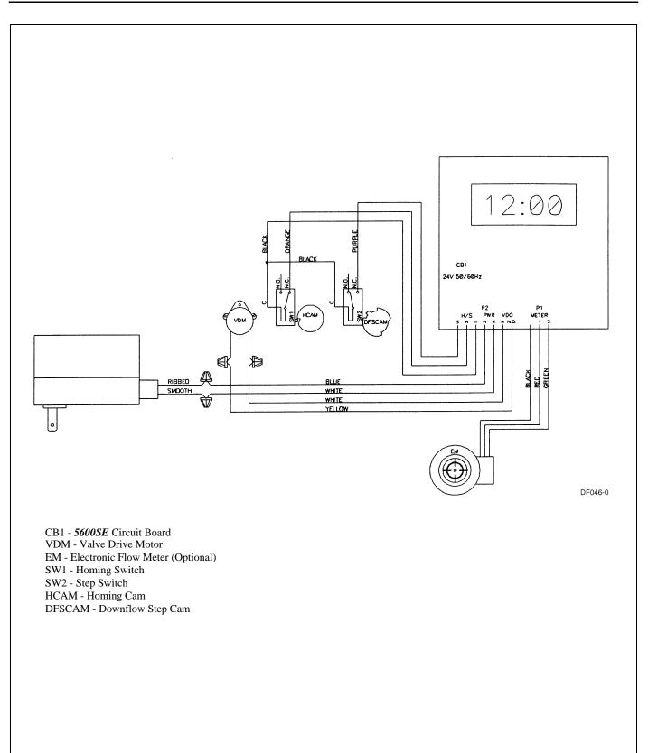
Figure 22: Valve Wiring Diagram
