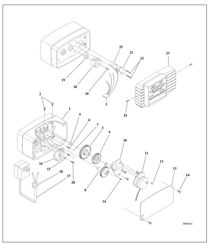
Figure 16: Valve Powerhead Assembly
