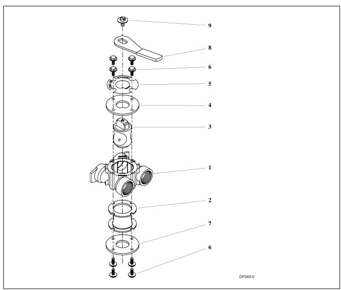
Figure 19: Bypass Valve Assembly, Brass
